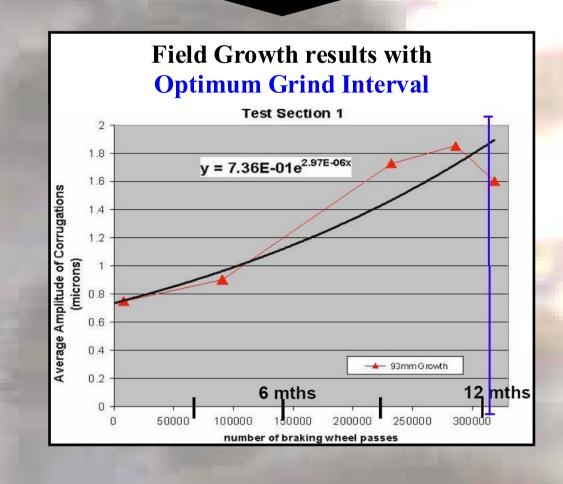
Development of a control system for the mitigation of rail corrugation, using growth estimator technol-
